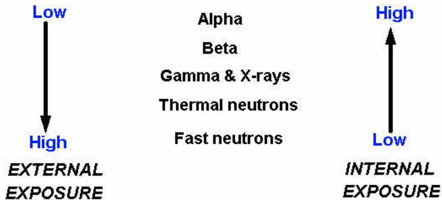
Figure 3. A diagram illustrating the relative risks from the types of radiation. The degree of risk depends on whether the exposure is internal or external.
